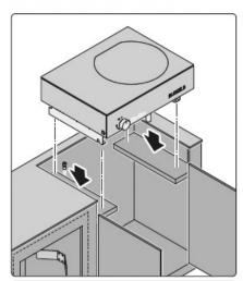
Place the appliance on the substructure.
